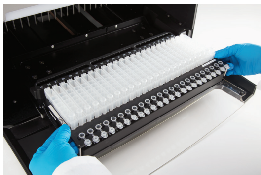
Figure 41. Placing the cartridges in the Deck Tray and pressing firmly to snap them in place.
