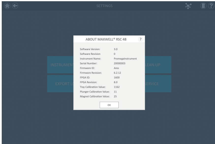
Figure 15. 'About Maxwell® RSC 48' screen. Instrument- and software-specific information is displayed on the 'About Maxwell® RSC 48' screen.
