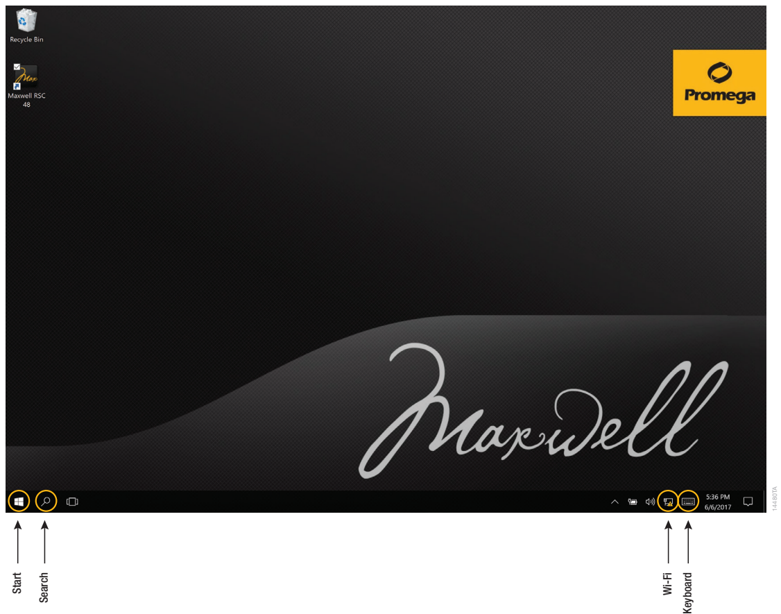
Figure 73. The 'Desktop' Screen. At the bottom of the 'Desktop' screen is the task bar. Access to the options and settings referenced in this document is provided by the Windows® Start, Search, Speaker, Wi-Fi and Keyboard buttons in the task bar.
