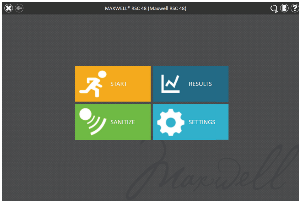
Figure 13. Maxwell® RSC 48 software 'Home' screen. The Instrument name appears in the title bar of the user interface.
