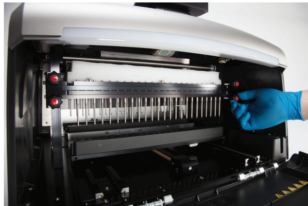
Figure 68. Placement of plastic stoppers. Move the magnet and plunger bars up, and secure the four shipping screws on both sides of the magnet and plunger bars.
