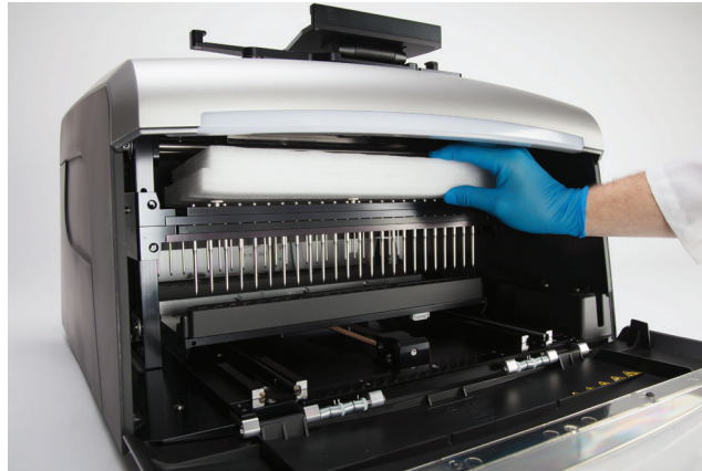
Figure 67. Placement of upper die-cut foam.
