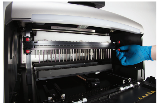
Figure 7. Removing the two foam pieces from inside the instrument. Panel A. Remove the front foam piece. Panel B. Remove the four shipping screws from the sides of the front magnet and plunger bars..
