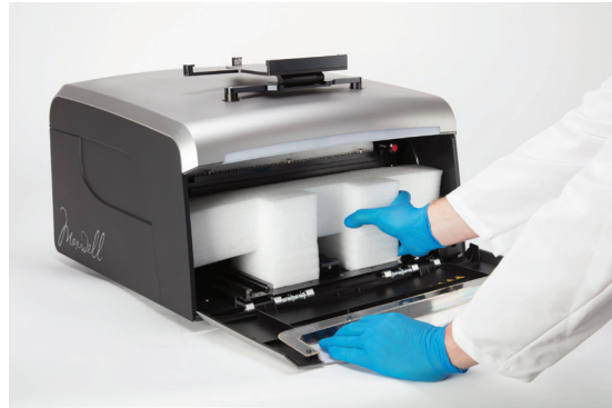
Figure 69. Insert the front die-cut foam. Make sure the serrated edge covers the magnet rods.
