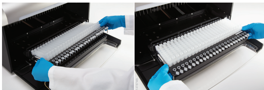
Figure 42. Placing the deck tray in the instrument.
