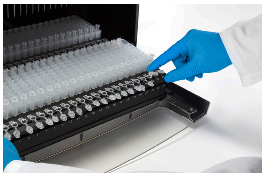
Figure 45. Closing the elution tube caps.
