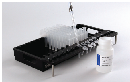
Figure 2. Setup and configuration of the deck tray. Nuclease-Free Water (50µl) is added to the elution tubes as shown.
